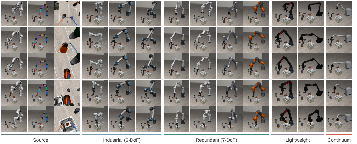
Fig. 3. BBQ-sauce-to-basket on Cross-Object (task 3). The first three columns show one Franka source demonstration and its front/wrist skeleton views. Target columns follow the robot order in Table I and show SkelWAM control replays from recorded states. Rows align initialization, approach, grasp, transport, and the LIBERO goal state across independently selected trials.
